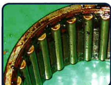
Bearing damage due to oil degradation
